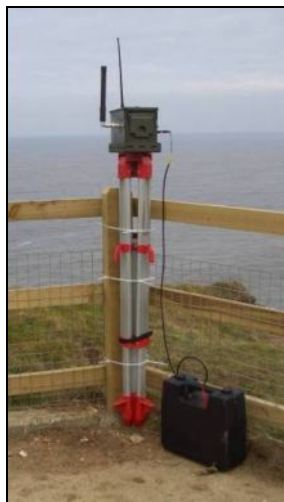
Figure 1: Main GPS jammer unit at Flamborough Head, shown with omni-directional antenna
